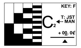
If the A4 MENU item is then changed to a non-default value (even if it is not saved) by pressing one of the MENU buttons to make A4 the "current MENU item" in the bottom text line and turning the VALUE rotary knob to display a value of, say, 440.5, then the non-default status of A4 will appear in its given position (second text line). These non-default status displays will persist even when a new "current MENU item" is selected:
