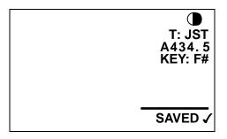
The VS-1 tuner would now power-on with these MENU item values until a new SAVE procedure is completed. The last entered tuning mode will resume when one of the MENU buttons is pressed to create a new "current MENU item" and exit SAVE mode.
