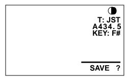
At this point, the current values of the four MENU items are displayed so that you can review the values you will be saving. Pressing either MENU button at this point will cause a new MENU item to become current and no saving operation will have occurred. By either turning the VALUE knob or pressing the **CHOOSE button** once, however, a "confirmation" screen will appear:
